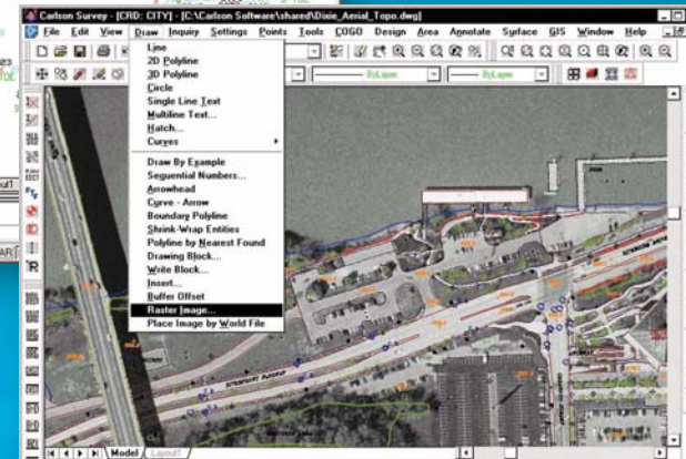
Imported raster images can be scaled and survey points and mapping drawn and plotted with the image
