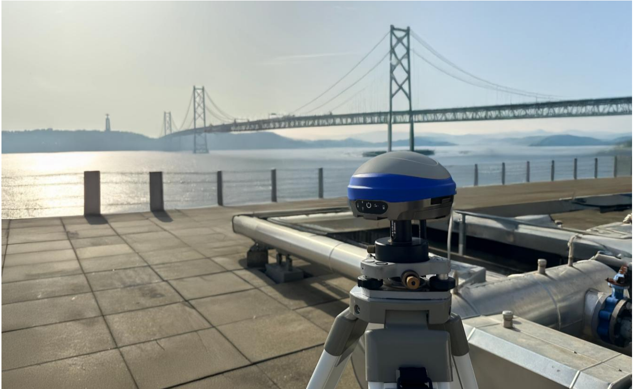
Figure 12 - Viking installed on a tribrach.
